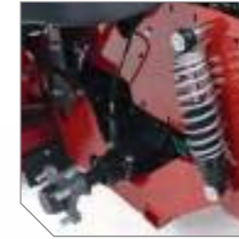
Suspension system with independent rear coil-over-shocks (shown) and pivoting front axle with front ride dampening shocks.
