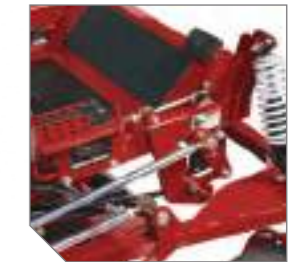
The foot-operated hydraulic deck lift system makes raising and lowering the deck effortless.
