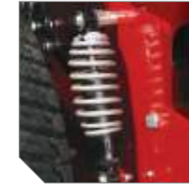
Patented suspension system consists of adjustable rear coil-over-shocks (shown) and front independent adjustable coil-over-shocks.
