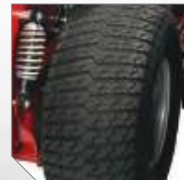
Large 26" drive tyres allow for greater traction, smoother ride and improved curb climbing performance.
