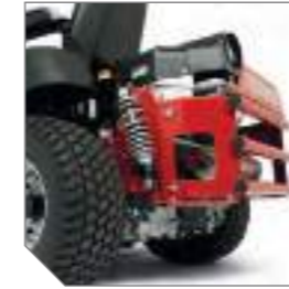
Rear suspension with coil-over-shocks and pivoting front axle with motion dampening shocks.
