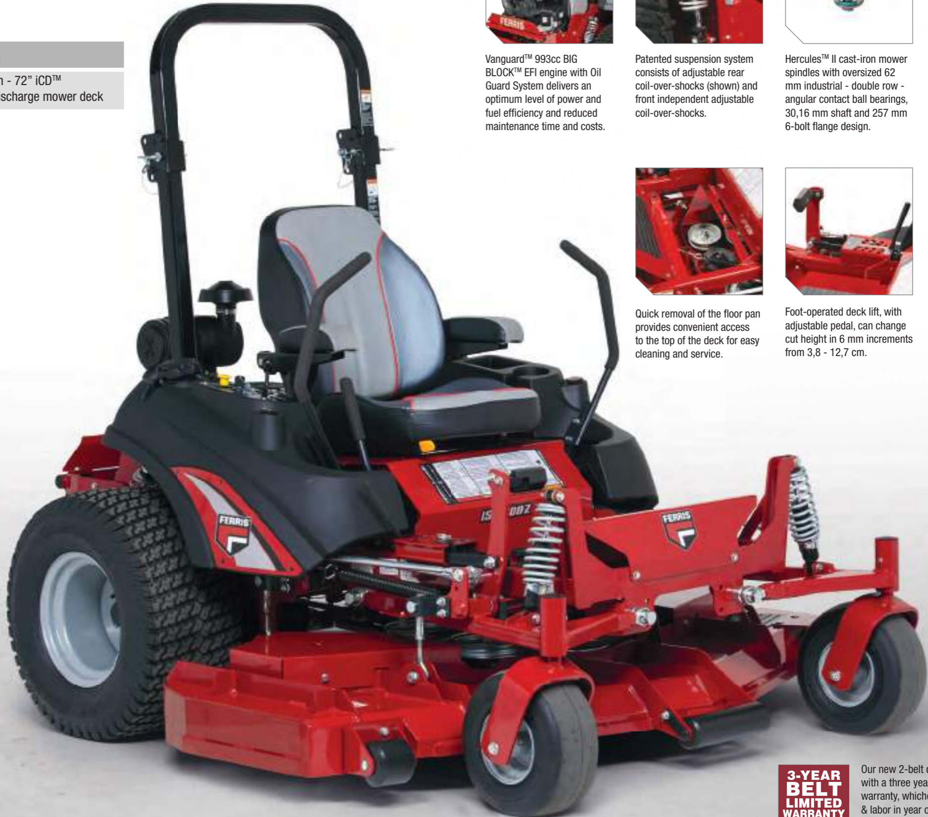
Dual, commercial Hydro-Gear ® ZT-5400 Powertrain ® transaxles deliver unmatched power and durability.
