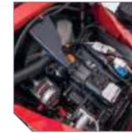
The efficient Yanmar™ 3 cylinder diesel engine (model 3TNM74F-SAFS) complies with the EPA Final TIER 4 emission regulation (Euro Stage 5 ready).
