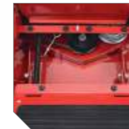
Removable floor plate provides convenient access to the top of the deck for easy cleaning and maintenance.
