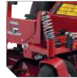
Suspension system consists of rear coil-over-shocks and front independent adjustable coil-over-shocks.
