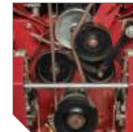
More than 180 degree belt wrap on drive system from shaft drive to flail rotor to ensure power transmission to rotor. Rotor drive powered by a bonded duplex belt.
