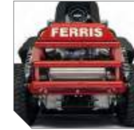
Heavy duty bumper protects the engine while also allowing for easy service access.
