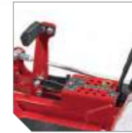
Foot-operated deck lift with adjustable pedal, takes the effort out of adjusting the cutting height.
