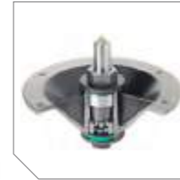
Hercules™ II cast-iron mower spindles with oversized 62 mm industrial - double row - angular contact ball bearings, 30,16 mm shaft and 257 mm 6-bolt flange design.
