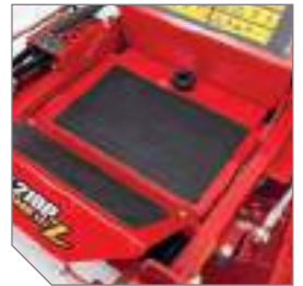
The floor plate of the IS ® 2100Z can be removed quickly shortening the time to service your mower properly.
