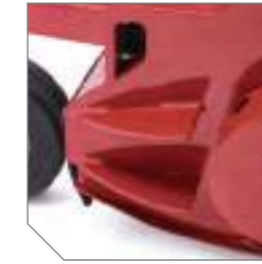
Impact protective guards to avoid damage to rotor bearings and belt drive system.
