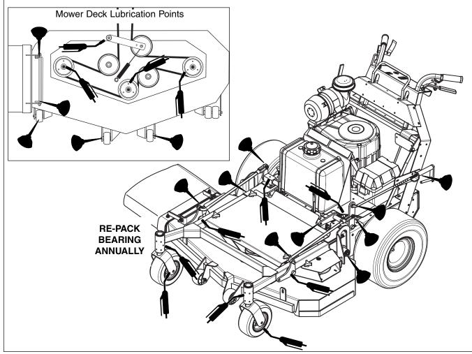
Figure 15. Lubrication Points
