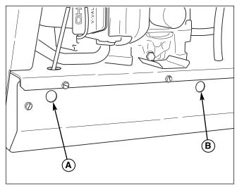
Figure 30. Neutral & Tracking Adjustment Points
