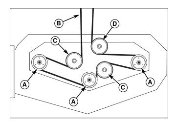
Figure 28. Mower PTO Belt Routing
