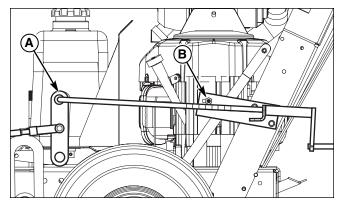
Figure 21. Deck Height Position A. Rear Deck Lift Rod Lever
