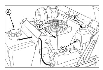
Figure 11. Fuel Tank, Oil Reservoir & Fuel Filter
