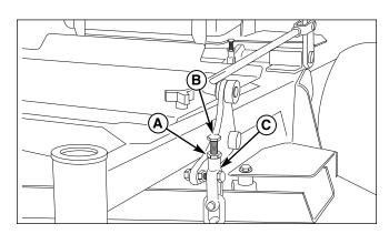
Figure 26. Deck Level Adjustment
