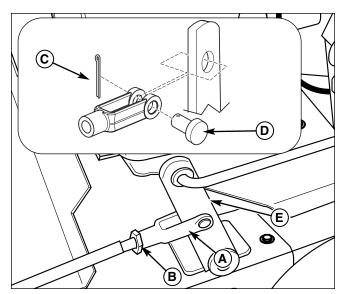
Figure 23. Lift Rod Clevis Adjustment
