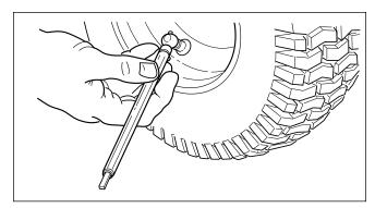
Figure 10. Checking Tire Pressure
