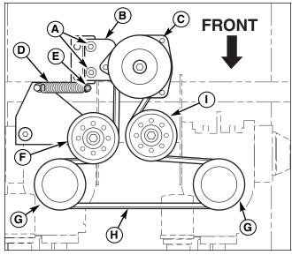
Figure 29. Transmission Drive Belt
