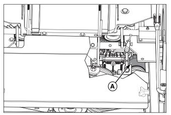
Figure 32. Transmission Oil Filter Location (left-hand side shown with deck guard cut away.)
