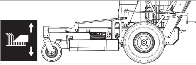
Figure 20. Mowing Height Adjustment A. Cutting Height Adjustment Handle
