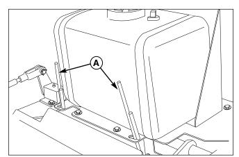
Figure 9. Hydraulic System By-Pass A. Hydraulic Release Levers
