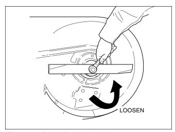
Figure 17. Removing the Blade
