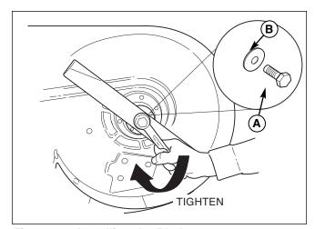
Figure 19. Installing the Blade A. Bolt
