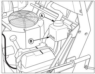
Figure 31. Oil Reservoirs A. Oil Reservoirs
