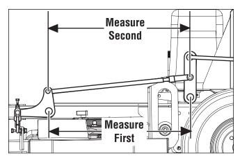
Figure 22. Measure and Adjust Deck Lift Rod Timing
