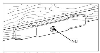
Figure 18. Balancing the Blade
