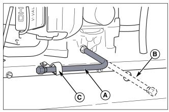
Figure 12. Engine Oil Drain
