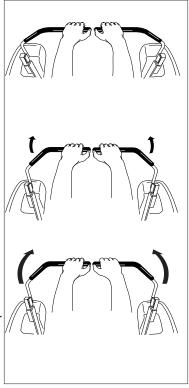
Figure 3. Move Control Levers Gradually
