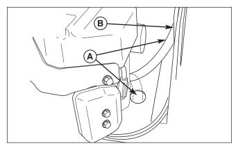
Figure 15. Engine Oil Drain A. Oil Drain Hose
