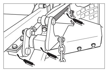
Figure 21. Deck Lift Linkage Pivots
