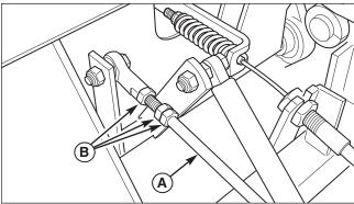
Figure 31. Neutral Adjustment (RH side shown)
