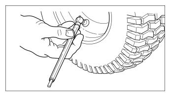
Figure 14. Checking Tire Pressure
