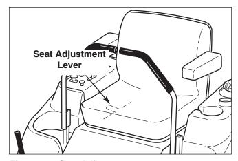
Figure 28. Seat Adjustment
