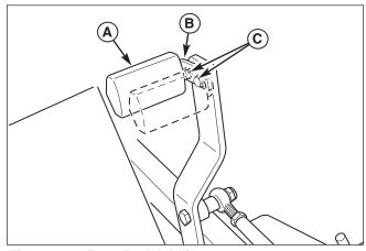
Figure 36. Foot Pedal Adjustment
