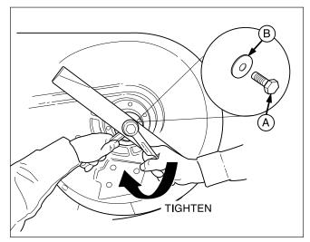
Figure 27. Installing The Blade A. Blade Bolt B. Flat Washer
