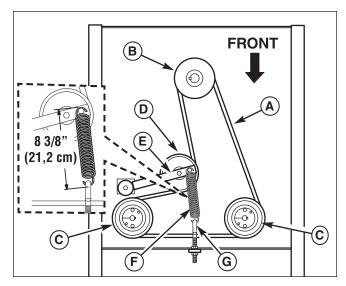
Figure 43. Hydraulic Pump Drive Belt Replacement
