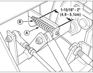
Figure 33. Parking Brake Adjustment
