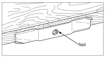
Figure 26. Balancing The Blade
