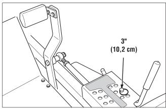
Figure 38. Deck Lift Pedal & Pin Position
