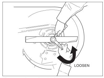
Figure 25. Removing the Blade
