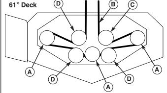
Figure 45. Mower PTO Belt Routing
