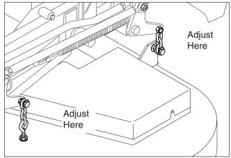
Figure 41. Hanger Chain Adjustment
