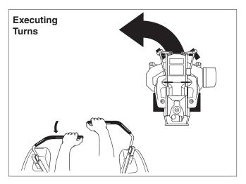
Figure 6. Turning Around a Corner
