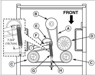
Figure 43. Hydraulic Pump Drive Belt Replacement
