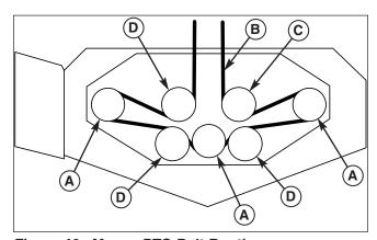
Figure 46. Mower PTO Belt Routing
