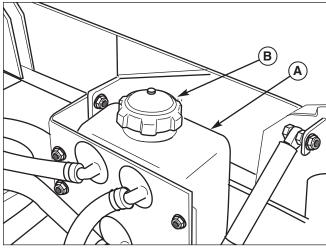
Figure 13. Checking Hydraulic Oil Level
