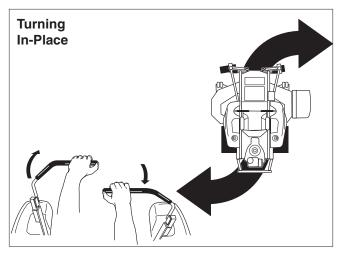
Figure 7. Turning in Place
