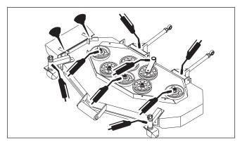
Figure 18. Deck Lubrication
