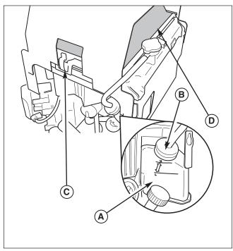
Figure 15. Radiator, Screen & Overflow Bottle
