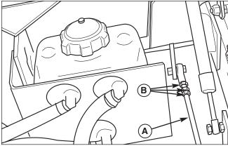
Figure 28. Neutral Adjustment A. Adjustment Linkage Rod B. Nuts
