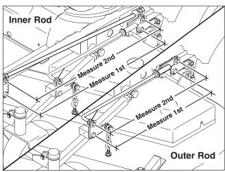
Figure 37. Measure the Inner & Outer Lift Rods
