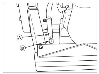
Figure 12. Engine Oil Drain A. Oil Drain Hose
