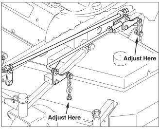
Figure 41. Deck Level & Spring Length Adjustment
