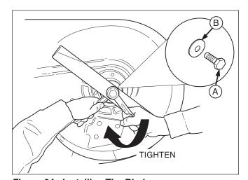
Figure 24. Installing The Blade
