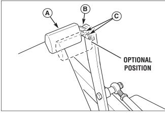
Figure 36. Foot Pedal Adjustment
