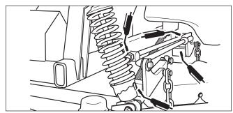
Figure 16. Deck Lift Linkage Pivots
