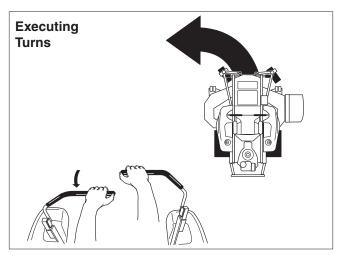
Figure 6. Turning Around a Corner
