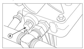
Figure 2. Hydraulic System By-Pass A. Hydraulic Release Valve (left-hand pump shown)
