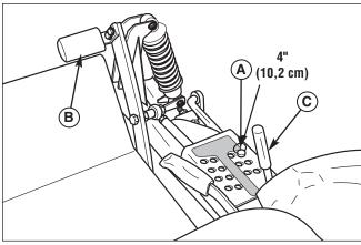
Figure 35. Cutting Height Adjustment
