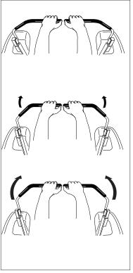
Figure 3. Move Control Levers Gradually
