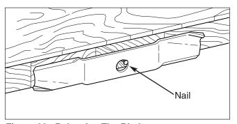
Figure 23. Balancing The Blade
