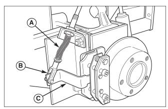
Figure 31. Parking Brake Adjustment
