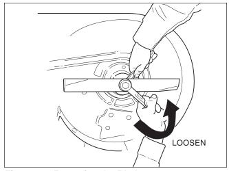
Figure 22. Removing the Blade
