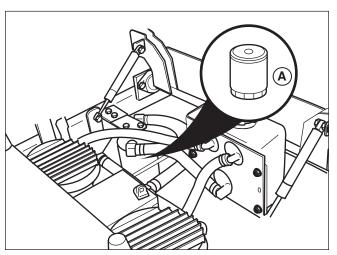
Figure 14. Hydraulic Oil Filter Location A. Oil Filter
