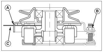
Figure 34. Adjust PTO Clutch
