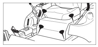
Figure 17. Control Handle Pivots
