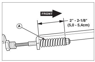
Figure 30. Parking Brake Adjustment A. Upper Brake Spring
