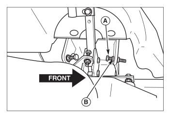
Figure 27. Top Speed Adjustment A. Top Speed Adjustment Bolt
