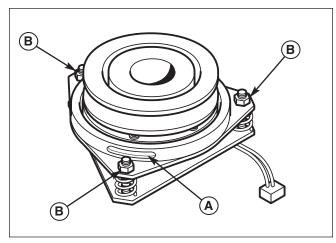
Figure 33. PTO Clutch Adjustment A. Adjustment Window (Qty. 3, one shown) B. Adjustment Nut
