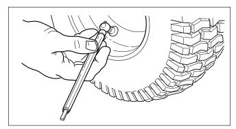
Figure 11. Checking Tire Pressure
