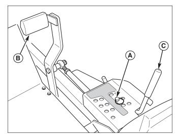
Figure 31. Mowing Height Adjustment A. Cutting Height Adjustment Pin
