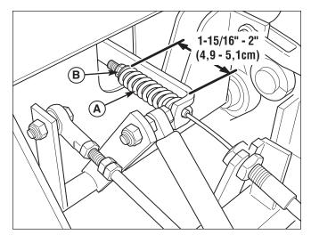
Figure 27. Parking Brake Adjustment A. Brake Spring B. Adjustment Nut
