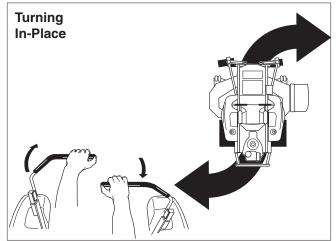
Figure 7. Turning in Place
