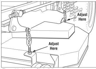
Figure 35. Hanger Chain Adjustment
