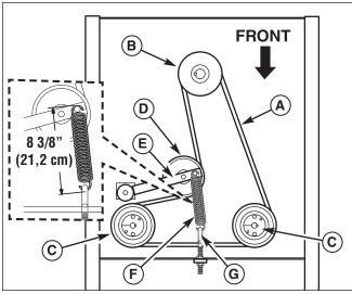
Figure 36. Hydraulic Pump Drive Belt Replacement
