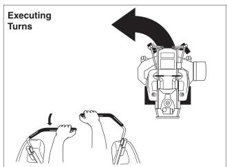
Figure 6. Turning Around a Corner
