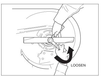
Figure 21. Removing the Blade
