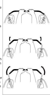
Figure 3. Move Control Levers Gradually
