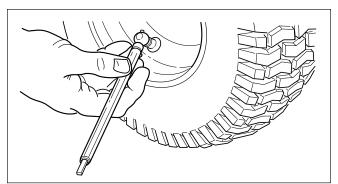
Figure 13. Checking Tire Pressure
