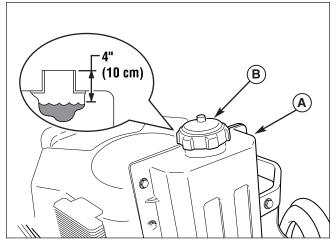
Figure 19. Checking Hydraulic Oil Level
