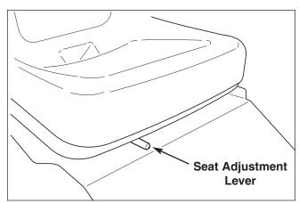
Figure 24. Seat Adjustment
