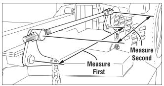
Figure 32. Check Lift Rod Timing
