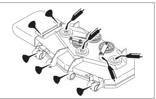
Figure 15. Deck Lubrication
