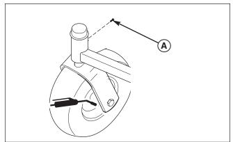
Figure 18. Front Caster & Wheel A. 1/4-28 Bolt
