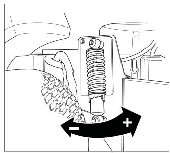
Figure 28. Rear Suspension Adjustments
