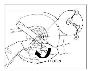
Figure 23. Installing The Blade A. Blade Bolt B. Flat Washer
