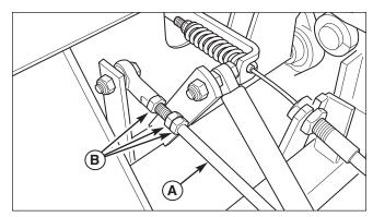
Figure 30. Neutral Adjustment (RH side shown) A. Adjustment Linkage Rod B. Nuts
