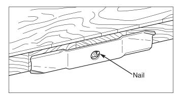
Figure 22. Balancing The Blade
