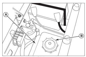
Figure 16. Hydraulic Oil Reservoir
