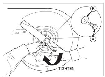
Figure 29. Installing The Blade A. Blade Bolt B. Flat Washer
