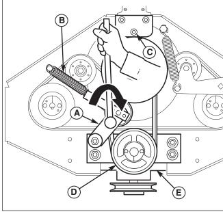
Figure 49. Clutch Belt Removal & Replacement
