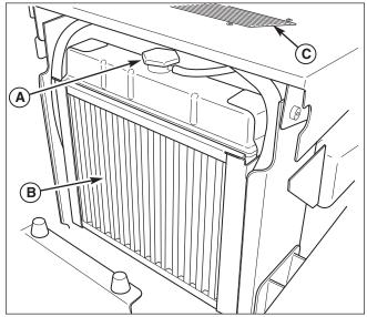
Figure 18. Radiator & Oil Cooler
