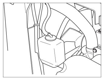
Figure 19. Radiator Expansion Tank
