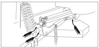
Figure 20. Deck Lift Linkage Pivots
