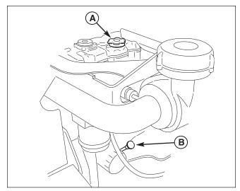
Figure 15. Change Oil & Filter A. Oil Fill Cap
