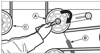
Figure 47. Mower PTO Belt A. Spring-loaded Idler Pulley
