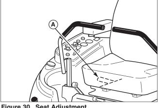
Figure 30. Seat Adjustment A. Seat Adjustment Lever
