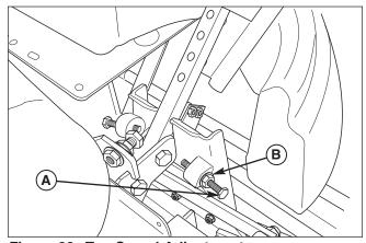
Figure 32. Top Speed Adjustment A. Top Speed Adjustment Bolt
