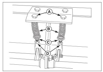
Figure 34. Neutral Spring Return Adjustment
