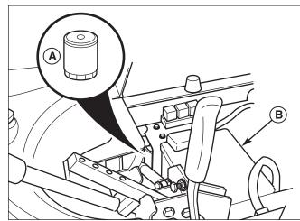
Figure 17. Hydraulic Oil Filter Location
