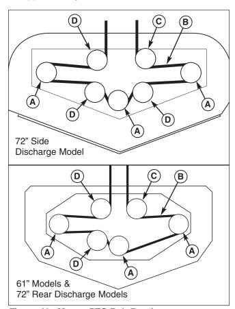
Figure 48. Mower PTO Belt Routing
