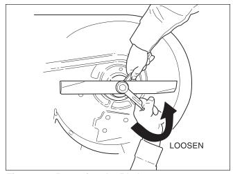
Figure 27. Removing the Blade
