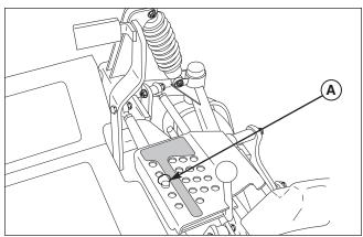
Figure 41. Deck Lift Pedal A. Height Adjustment Pin
