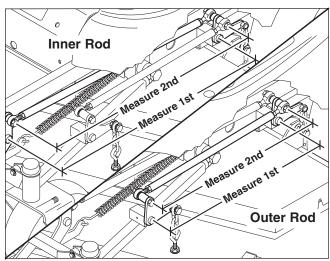
Figure 40. Measure the Inner & Outer Lift Rods
