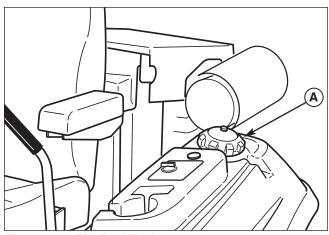
Figure 13. Fill Fuel Tank A. Fuel Cap
