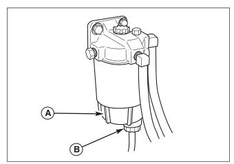
Figure 14. Drain Fuel Filter A. Fuel Filter Bowl
