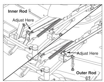
Figure 42. Adjust the Inner & Outer Lift Rods
