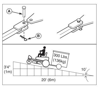
Figure 10. Trailer Weight Recommendations A. Clevis Pin B. Clip
