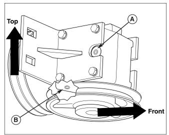
Figure 51. Gearbox Oil Level A. Fill Plug B. Drain Plug
