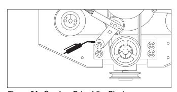
Figure 24. Gearbox Drive Idler Pivot
