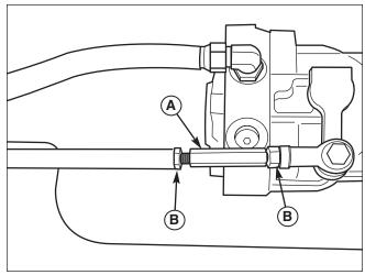
Figure 33. Neutral Adjustment (Left-hand side shown)
