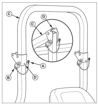
Figure 11. Raise & Lower the Roll Bar
