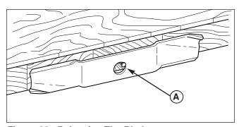
Figure 28. Balancing The Blade A. Nail
