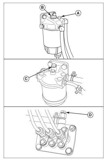
Figure 2. Fuel System Priming
