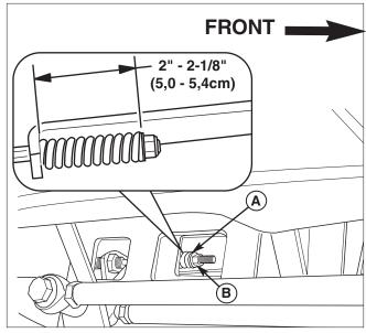
Figure 35. Parking Brake Adjustment A. Upper Brake Spring B. Adjustment Nut
