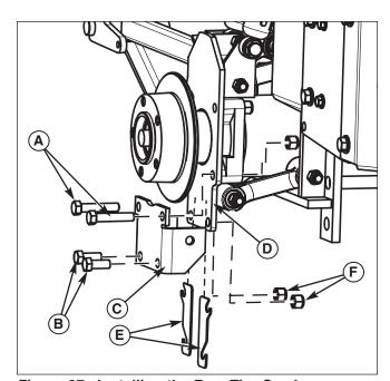
Figure 37. Installing the Rear Tire Camber
