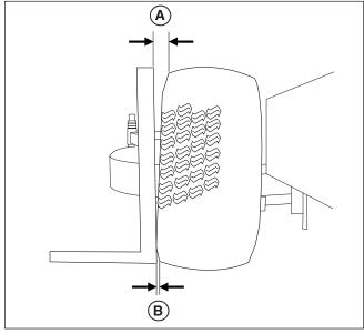
Figure 36. Measuring the Camber Distance A. Top Measurement
