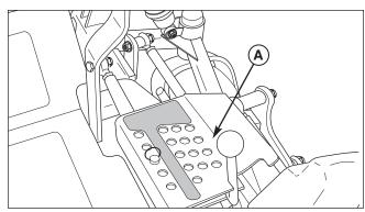
Figure 46. Lower the Mower Deck A. Height Adjustment Pin
