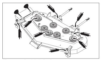
Figure 21. Deck Lubrication
