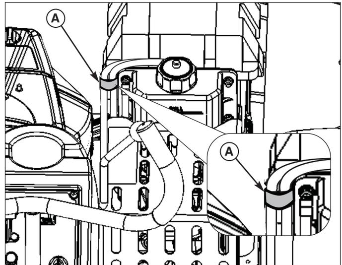
**Figure 1. Inspect for Vinyl Hose Clamp
