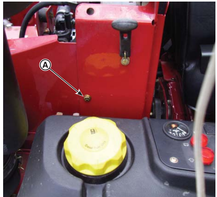
Figure 1. Removing the Radiator Shroud Hardware
