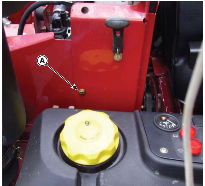
Figure 1. Removing the Radiator Shroud Hardware
